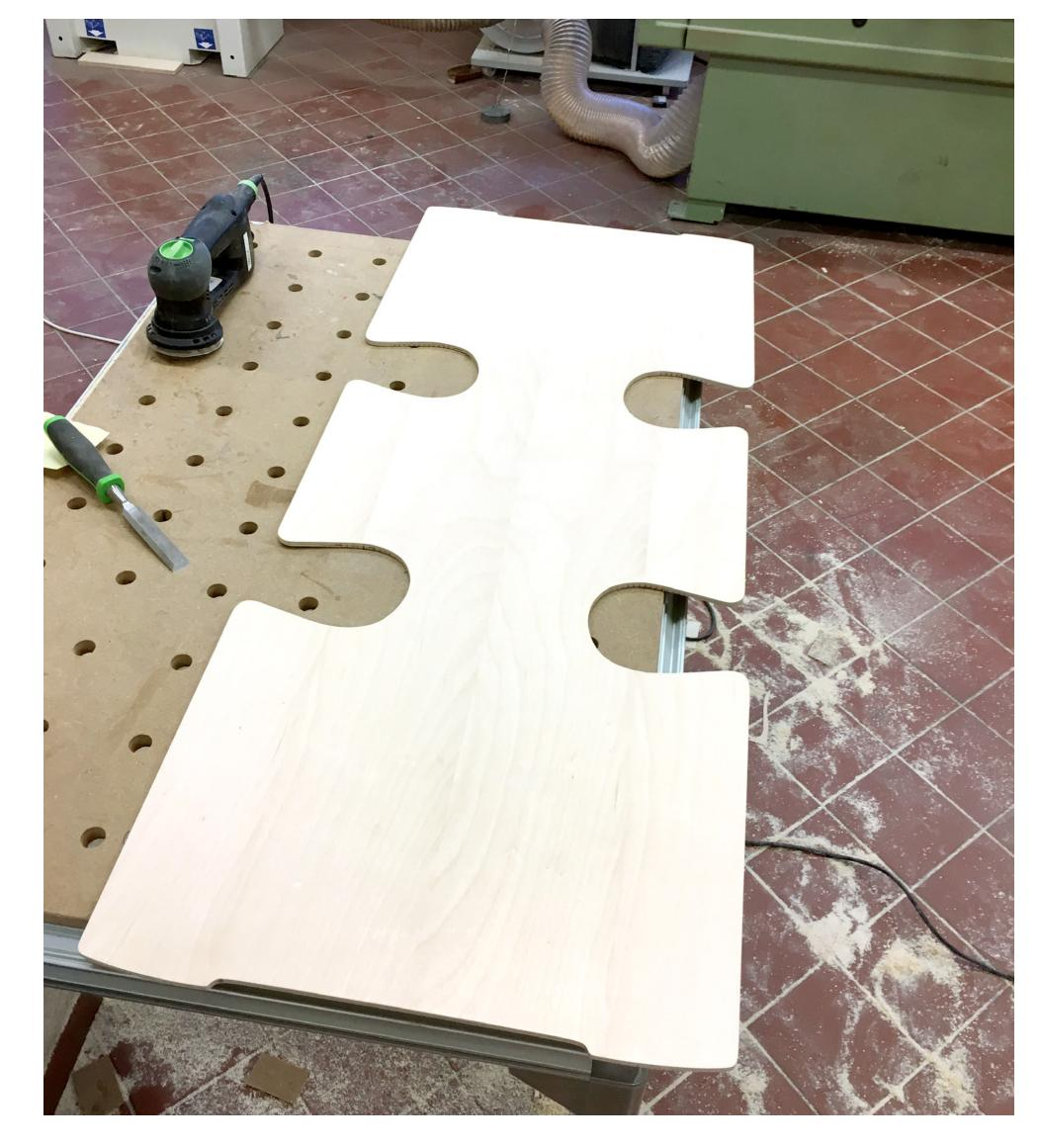
To bend or not to bend. Thanks to areas with trapeze-shaped strips on the inside, this plywood is easy to bend, yet impossible to crack—perfectly flat for shipping and storing.
